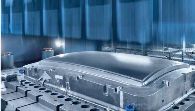
ZM Ecoprotect®-coated sheet displays excellent deep-drawing behavior.
