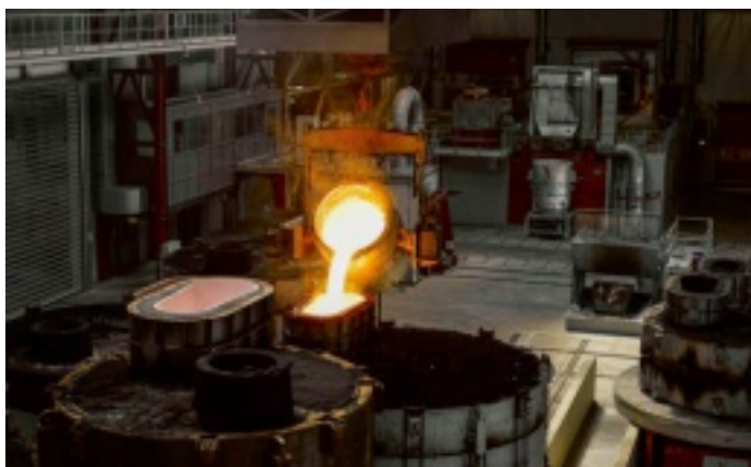
At the foundry in Georgsheil in the district of Aurich, Enercon recycles steel scrap from generator production. thyssenkrupp Steel helped to make this possible by optimizing the mix of materials used to produce its steel.
