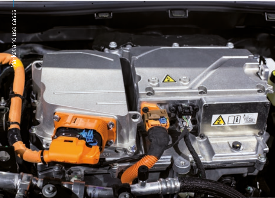
A cover made of bondal® can significantly reduce noise emissions from the inverter.
