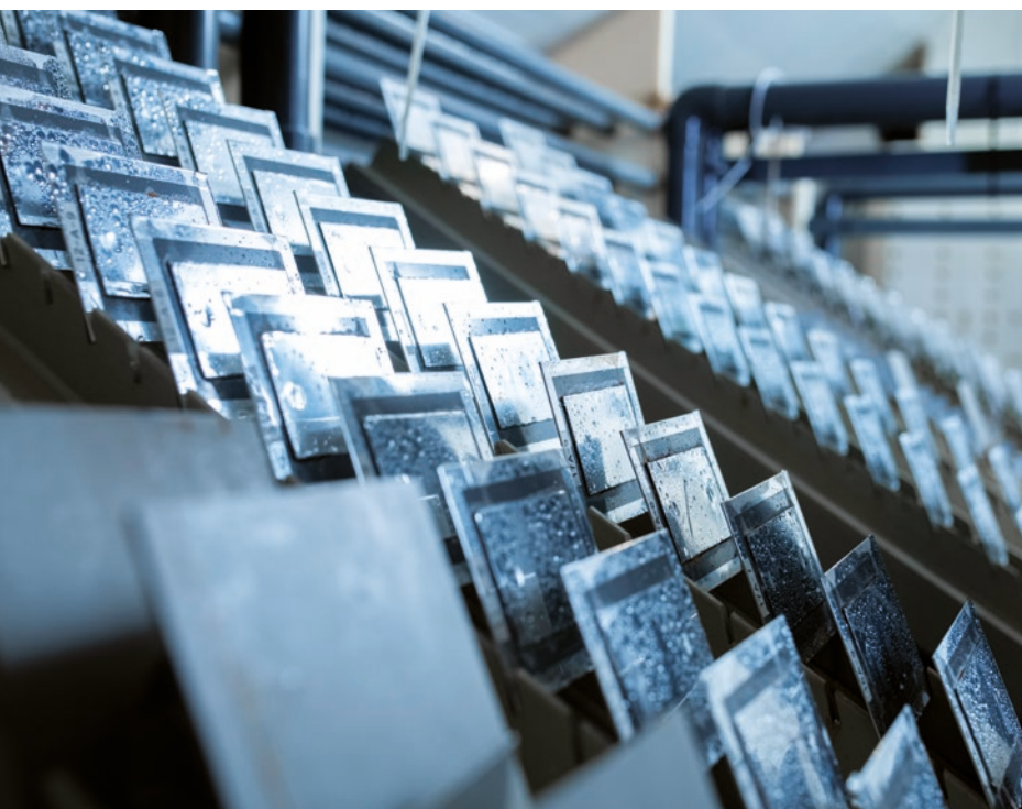
In thyssenkrupp Steel’s test chambers, different weather conditions are simulated for testing material samples.
