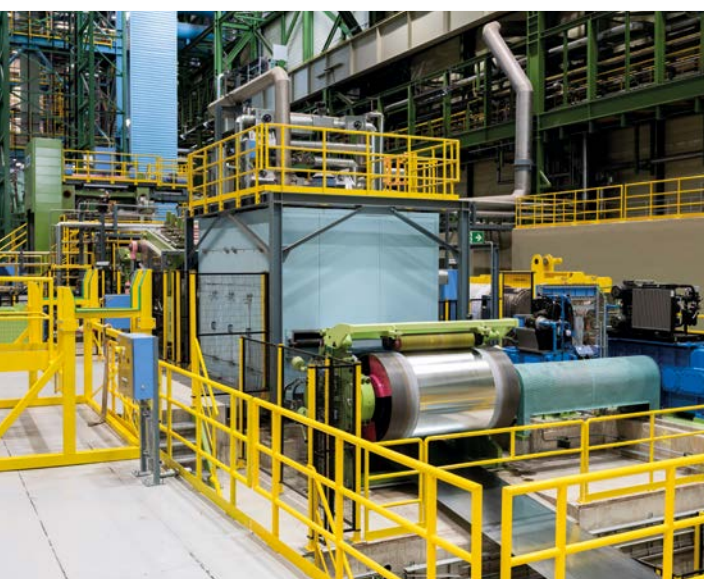
The line applies high-quality zinc coatings to the steel strip: pure zinc and zinc-magnesium coatings, such as ZM Ecoprotect®.
