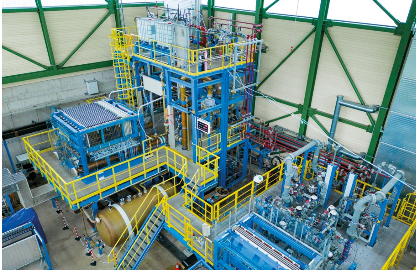
Pilot-scale electrolysis for hydrogen production: Carbon2Chem technical center in Duisburg supports further refinement of electrolysis for the production of green hydrogen.
