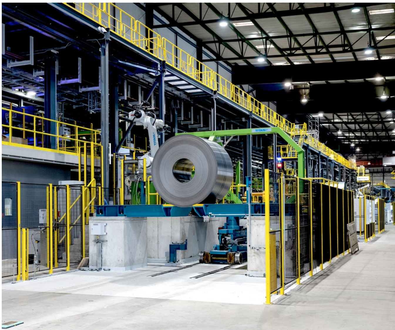
One of the two core units at thyssenkrupp Steel's new center of excellence for electric mobility in Bochum: the new Annealing and Insulation Line (AIL).
