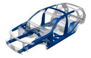
Front Side Member Rear Side Member Rocker/Side-sill Outer Seat Cross Member A Pillar Applications B Pillar Applications
