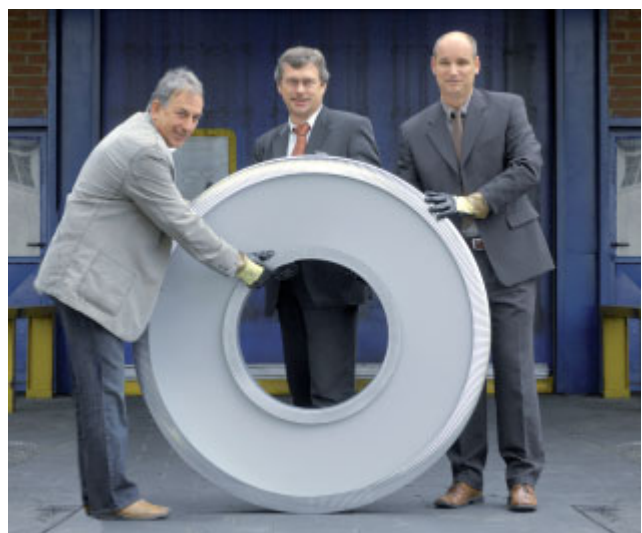
▼ If packed correctly, the coil will not suffer any scratches. Neurapack customer consultant Jürgen Schroller (left), Matthias Janz (middle) and Burghard David pictured with a coil that is fully protected by inner and outer edge protectors as well as a thin sheet blank on the sides.
