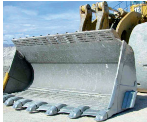
▶ Wear-resistant XAR® steel is used in construction machinery. This permits a longer service life and gives the customer significant cost advantages.
