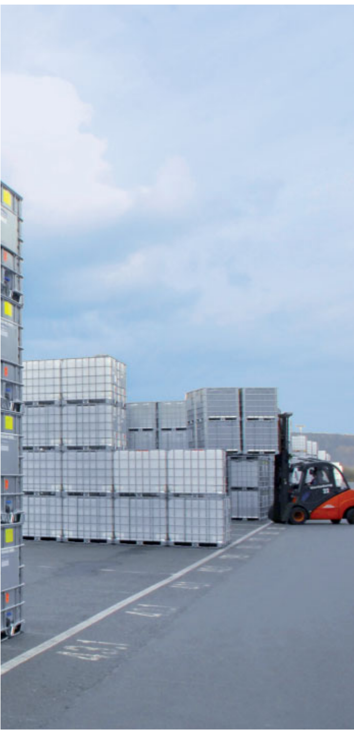
◀ The intermediate bulk container, IBC for short, is the major specialty of the Schütz Group. A steel cage houses the plastic insert that holds the goods, however a complete steel jacket can be used depending on the sensitivity of the material being transported. The containers offer the right quality for global clients who place great value on safety and cleanliness.
