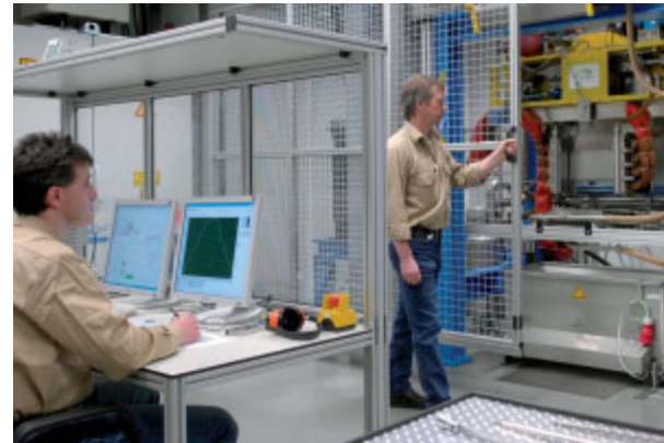
▲ Stefan Majewski (l.) and Volker Becela working with the new "Multipas" annealing simulator, which is installed in a cage for protective reasons. It only functions when the mesh doors are locked. The room is air-conditioned since the temperatures generated in the trials are very high.
