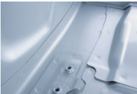
◀ The side member: Thanks to new plant technology at ThyssenKrupp Tailored Blanks in Duisburg-Hüttenheim, the blanks that arrive at Audi are already totally prepared for immediate direct hot stamping.
