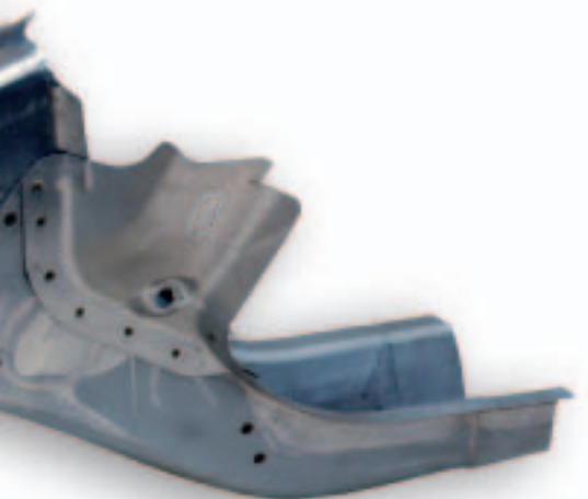
Weight reduced by 27 percent, costs down by 13 percent, 126 kg less CO 2 over the vehicle life. A longitudinal member based on the T 3 technology developed by ThyssenKrupp Steel Europe.
