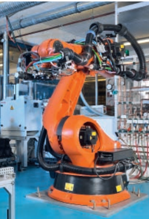
Welding robots in the 1,200 square meter Inpro test shop – for welding of body parts made of steel by ThyssenKrupp Steel Europe.
