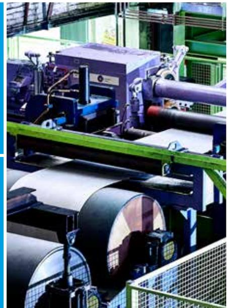
The process begins with the pickling of the hot strip. The aim is to remove the scale formed during hot rolling in a continuous pickling line. At the entry end, the front and tail ends of the hot rolled coils are welded together. In the form of a continuous strip they then pass through four working tanks, each 25 meters in length and built in turbulence design.
