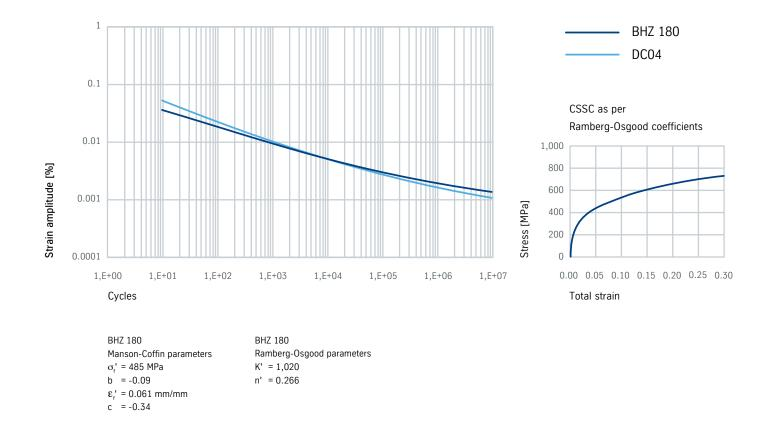
Stress-strain curve of a bake-hardening steel BHZ 180 compared to a deep-drawing steel DC04
