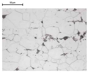
The picture shows the typical microstructure of a bake-hardening steel after etching with nital, with perlite and isolated granular cementite in the ferritic matrix.
