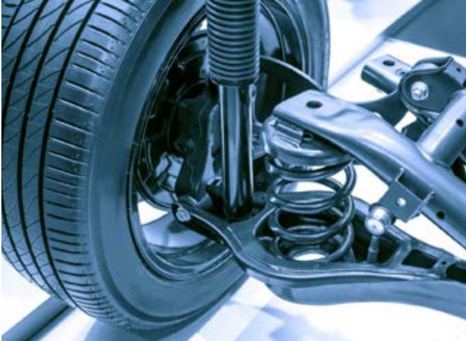
Highly ductile micro-alloyed steels for suspension components.
