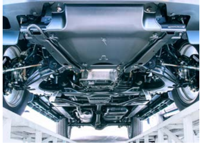
Highly ductile micro-alloyed steels in the chassis: In the area of axles or wheel suspension, for for subframes, cross members and side members.
