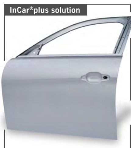
① Lightweight Litecor door, sandwich structure 0.25/0.40/0.20 mm
