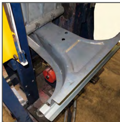
4 Dynamic three-point bending test setup (left), Tribond 1400 without failure (right)
