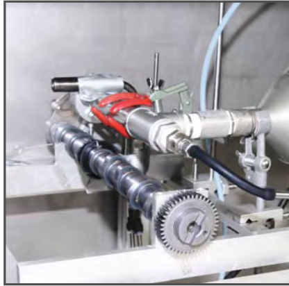
④ Laboratory test rig for determining the fraction and overall separation level as well as pressure loss
