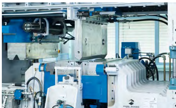
③ T 3 press adapter: springback-free holding of the U-shaped shell through displaceable walls
