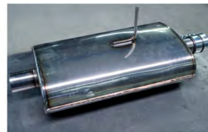
④ The prototype intermediate pipe (left) and muffler components for cyclical full load/no load tests (right)
