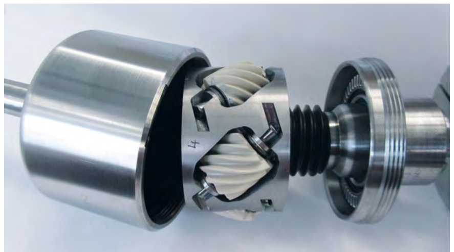
3 Superimposing actuator transmission with plastic gears
