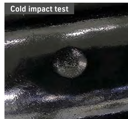
④ Impact crater without paint delamination
