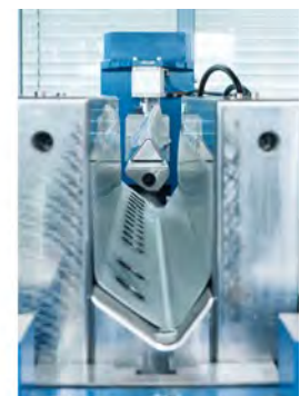
③ T 3 press adapter: springback-free holding of the U-shaped shell through displaceable walls
