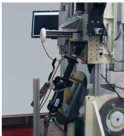
9 InCarplus solution in the drop tower crash test
