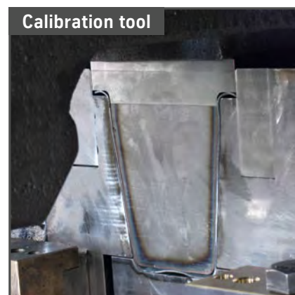
⑤ Structure of the calibration tool (left), calibration of the U-shaped shell with welding flange (right)
