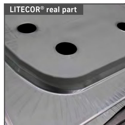
③ Comparison of the simulation (left) and component (right) in a critical forming location
