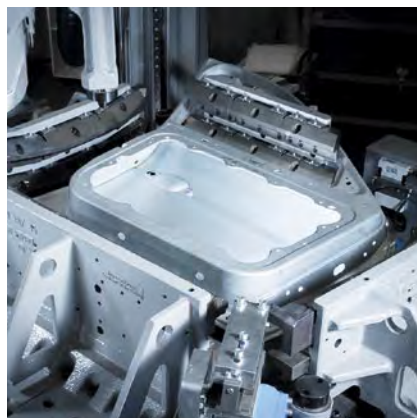
5 Mechanical hemming system and process steps
