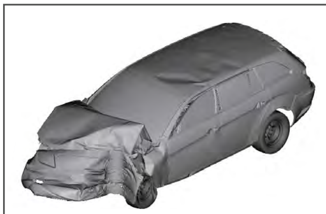
⑤ Litecor firewall intrusion after Euro NCAP frontal crash
