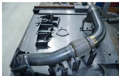
④ The prototype intermediate pipe (left) and muffler components for cyclical full load/no load tests (right)
