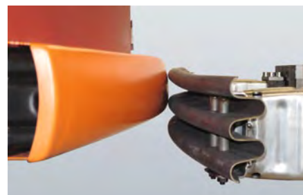
❸ Results of the RCAR bumper test crash simulation; cross-section with boundary level and test setup
