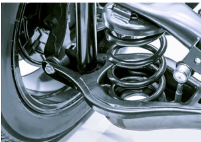
Highly ductile microalloyed steel for wheel chassis parts.
