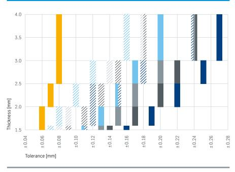
Thickness tolerances of hot-dip galvanized steel in comparison – normal and
